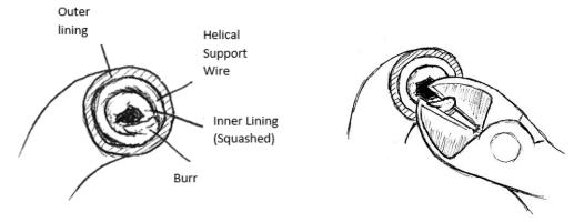
3. Carefully file any remaining protrusions, without getting the filings into the brake housing.
