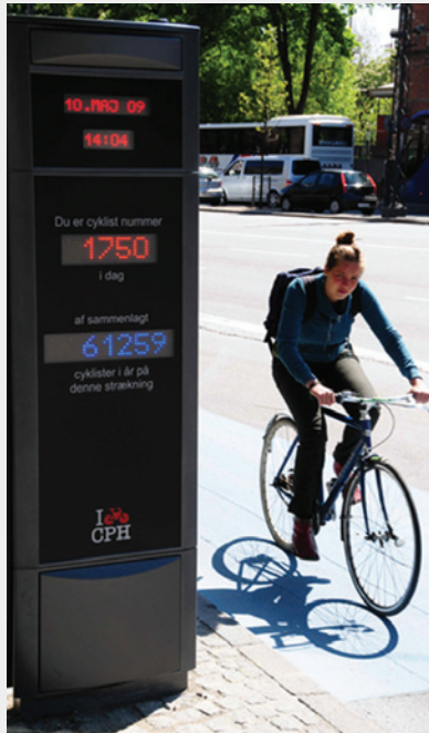
FIGURE 3.2.4 - AUTOMATED BICYCLE COUNTER IN COPENHAGEN, DENMARK
