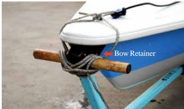
5. Place the bow of the boat onto the curved plastic bow retainer, and then secure the boat using the painter with a series of half hitches. Please see intermediate knot section of the manual for instructions on how to tie a half hitch.
